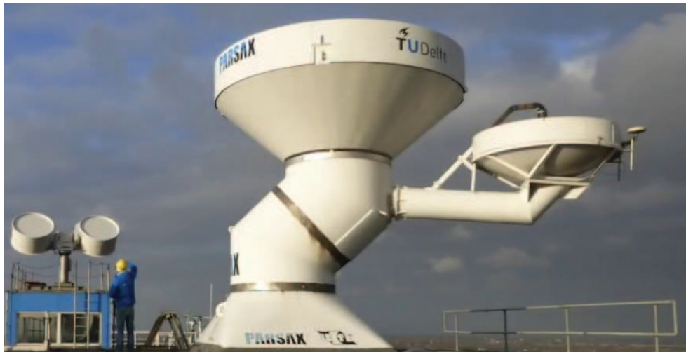
Figure 1. PARSAX radar (in front) and MESEWI radar (at the back)
